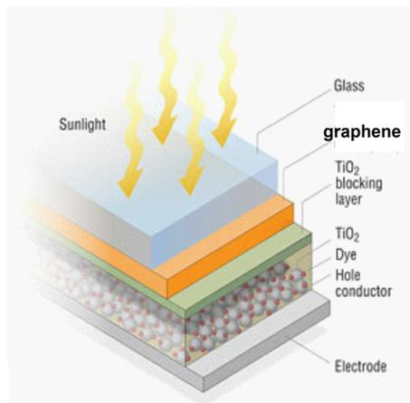
**Figure 3** – Sketch of a Dye Sensitized Solar Cell with graphene TCE
