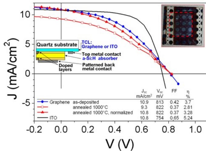
**Figure 2** - JV characteristics under AM1.5 illumination of a-Si:H pin solar cells integrating graphene as TCE. The data of the reference device are also included. Insets: sketch of the structure and picture taken on as deposited and annealed samples. The colored dashed square indicates the region covered by graphene
