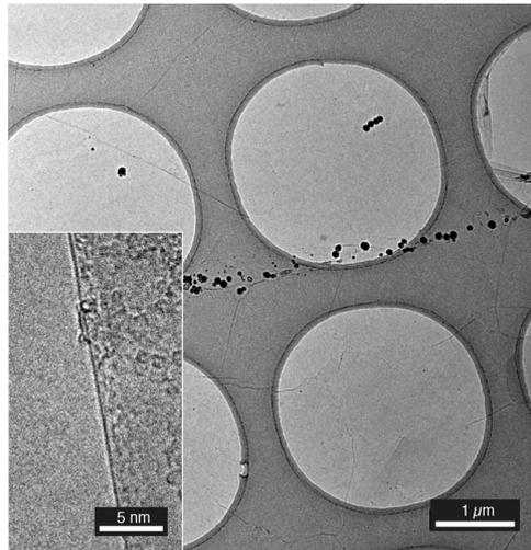
**Figure 1** - TEM image of a graphene membrane. The graphene spans over the whole 3 mm grid, covering the holes of the grid carbon film. (inset) Detail of a folded edge in a monolayer region.
